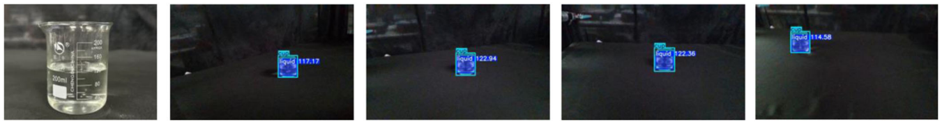
FIGURE 8 | Liquid volume estimation results for different viewpoints in real experiments. [Color figure can be viewed at wileyonlinelibrary.com ]
